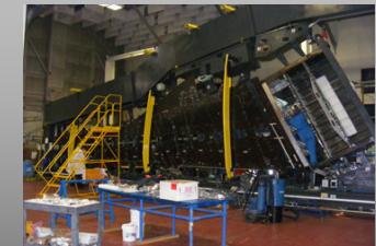
Monolithic structures using resin transfer methods
