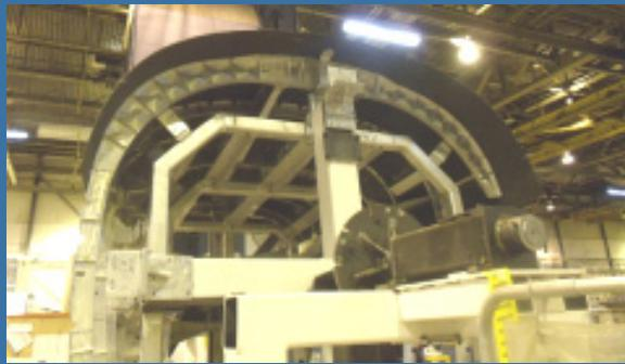
First Cockpit Center Post test piece
