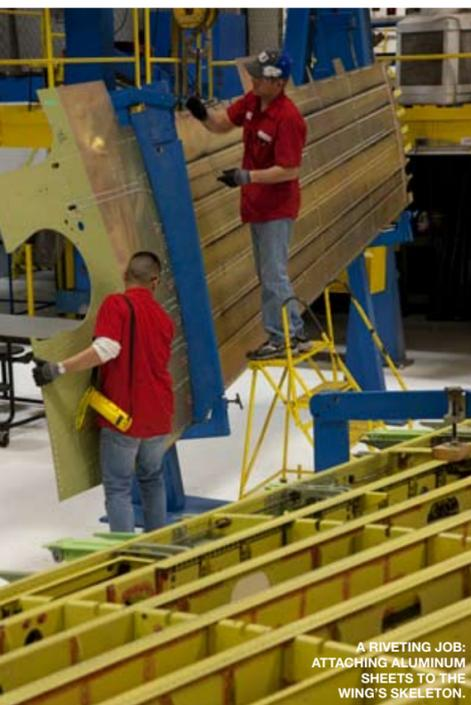
A RIVETING JOB: ATTACHING ALUMINUM SHEETS TO THE WING'S SKELETON.
