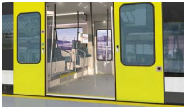
The OMNEO train offers maximum modularity. All doors offer level entrances adaptable to platform heights of 550, 760 or 920 mm.
