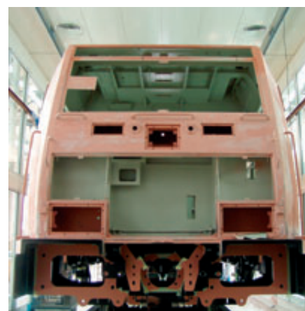
Environmental module "Common": Bombardier crash-optimised driver cabin in paint shop in Wroclaw.
