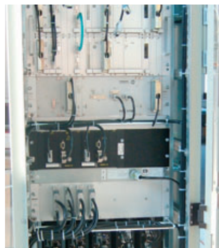
Env. module "Country": ETCS cubicle Bombardier * EBI* CAB 2000 with electronic Bombardier * MITRAC* CC
