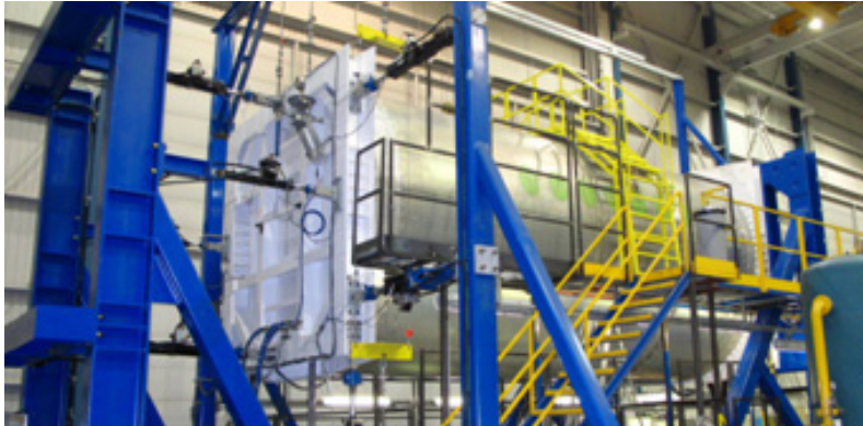
Center barrel tested for first life (60,000 flight cycles)
