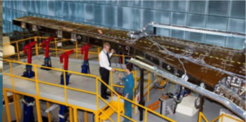
Composite wing demonstrator testing started in March 2010
